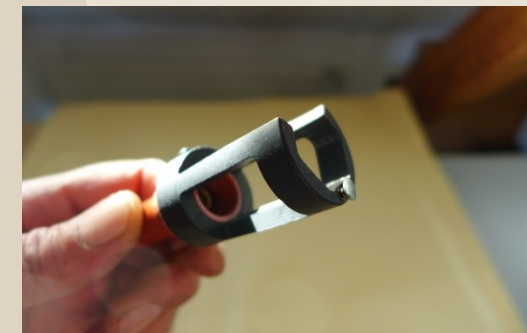
The temperature sensor is one unit with the spark plug connector. Changing plugs like always.
