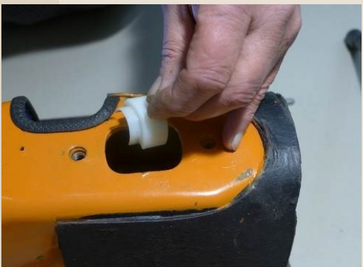
complete installation through the opening of the dismantled shifter. Gear selector rod keeps in
