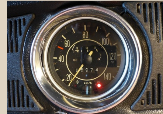
If temperature is reached, the oil pressure lamp starts flashing. Oil pressure function still working (double function)
