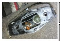
**1. Shifter out**. Do a mark where the parts are located. The assembling after installation is **not** part of the manual
