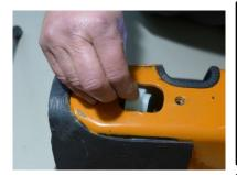
**6. Take the second half** with the hole in the same way. Put some grease on it. Push it in the shackle. Listen that both parts are in one line and fits.
