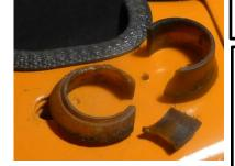
**3. take out the rest** of the old shifter bush. There is no really "best way" to do it. The spring ring can be taken out by a wire-cutting pliers. Pull hard. Clean the rod and the shackle from old grease and rests.
