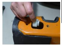
**4. Take the part with the slot** by the small screw. Put some grease on the bush. The only need of this screws is a better handling. Locate it in top of the rod and push it inside the shackle. The slot must be inside the shackle
